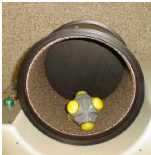
The Hexapod Drum is used for accelerated fatigue testing of carpet
